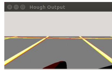
Figure 9: Result of Probabilistic Hough Transform
